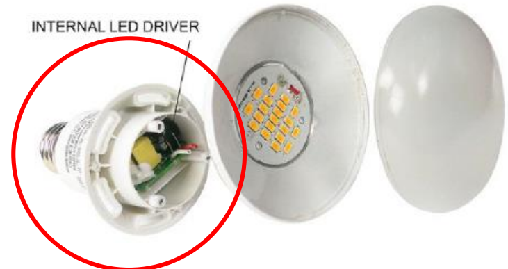
Diskrete LED source incl. separate LED element & electronic driver
