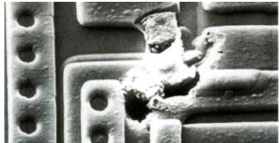
Damages to the I/O stages of ICs (they are often caused by ESD)
