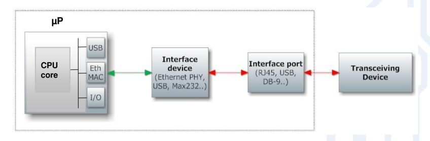
Test connections between  $\mu P$  / peripheral controllers and connected peripheral logic (at-speed)
